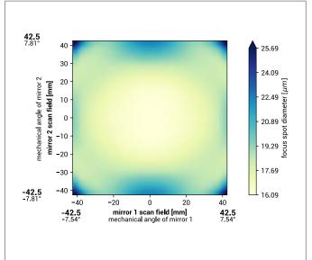
spot diameter at 86.5% level for a Gaussian beam (M² = 1) with 15.0 mm diameter at  $1/e^2$ , clipped at 15.0 mm field size and mirror distances as given above for a two mirror scan system
